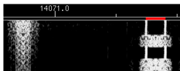
Figure 6.70: PSK Waterfall X4 scale
