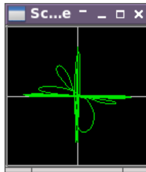
Figure 2.138: Classic RTTY XY Scope
