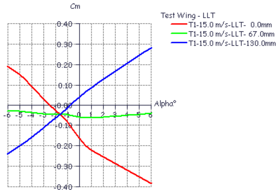
Figure 30: Wing Neutral Point
