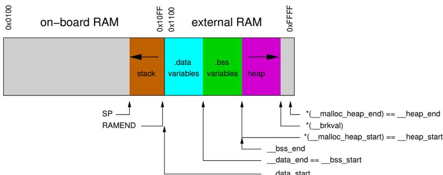
Figure 2: Internal RAM: stack only, external RAM: variables and heap
